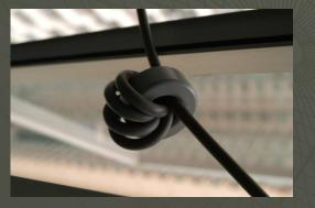
• #73 and #75 ferrite material work well at HF, and #43 and #61 at VHF
