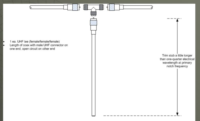
Open circuit at stub's end
