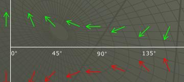
Short circuit: Reflected voltage is *out-of-phase* with incident voltage.
