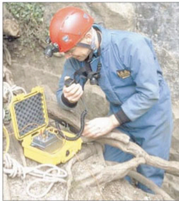
A HeyPhone in use on the surface above Carleswalk Caverns in Derbyshire.
