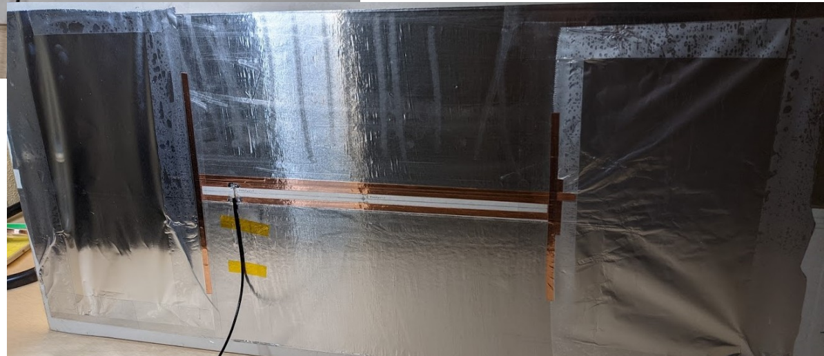
Textbook slot \lambda \times \lambda/2 Aluminum sheet \lambda/20 -fed
