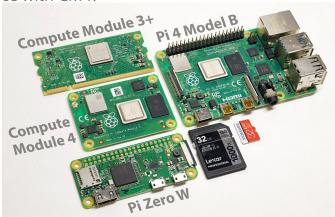
Raspberry Pi Compute Module is a RPi without the usual connectors. Instead it has some sub-micro cell-phone-internal-type connectors. It's meant for custom use cases like industrial and IoT.
