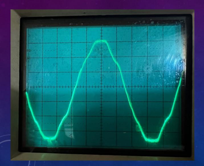
Modified sine wave, uneven slopes
