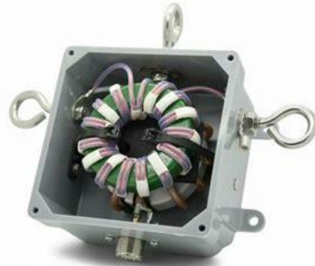
A 1:1.5 UNUN in series with a 75 \Omega choke (top)
